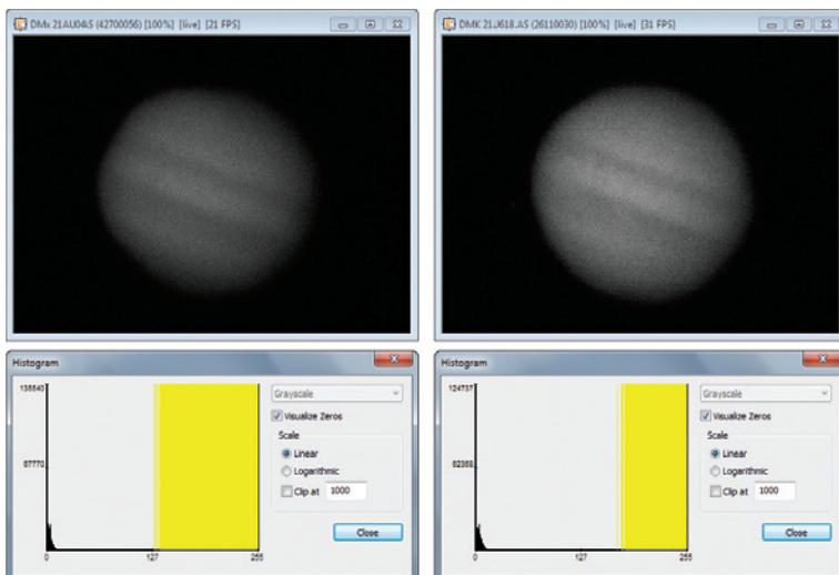
Though physically identical to its predecessor, the Imaging Source's new DMK 21AU618.AS video camera is significantly more sensitive, especially at the red end of the spectrum. These back-to-back recordings of Jupiter made through a red filter and the author's 12½-inch reflector show that the old camera (*far left*) produces a fainter image and less data as indicated by the greater portion of the histogram showing zeros (yellow area).
