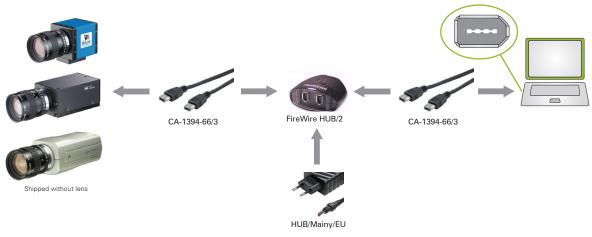
Laptop **does not** supply the FireWire socket with power
