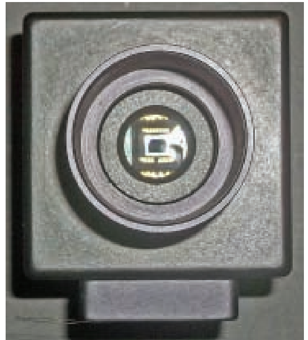
▲ The DMK 21AU618.AS' ICX618 chip is small in comparison to many DSLRs or CCDs for deep sky imaging, but is perfect for planetary imaging at 640 × 480, and can operate at up to 60 frames per second. Image: Nick Howes.
